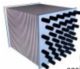
▲ Typical Plate-Fin Construction
